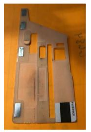
A **shimming device** (photo attached from one recently found on a credit union owned ATM) can be very difficult to detect. The slim card-shaped device is wedged or shimmed into the card reader which allows it to read each card that is inserted into the machine.
